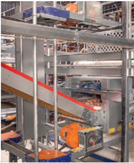
Egg collection with a vertical conveyor and automatic system egg collection by means of an elevator
