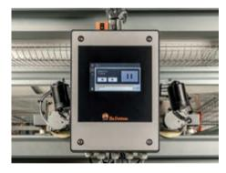
The 507 controller with its large display is the core of VIM. The farmer can configure all settings at this controller and read the scanned results.
