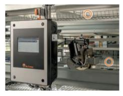
In each tier, the laser scans at the height of the birds' legs. VIM registers any larger obstacle. If this obstacle is still detected after a total of four scans per day, the probability of VIM having located a dead bird is very high.
