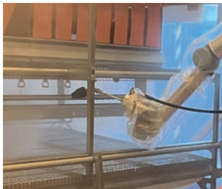
Inside and outside cleaning of the feed trough
