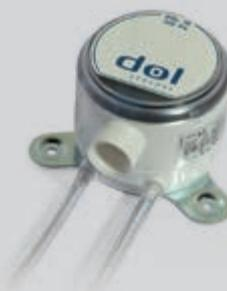
DOL 18 is a negative-pressure sensor that measures the pressure difference between inside and outside air. It emits a 0-10 V signal. Power for this sensor is supplied by ViperTouch.
