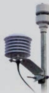
The DOL 58 weather station allows local weather conditions to be included in the ventilation control calculations. Wind direction, air speed and air pressure are measured for this purpose.
