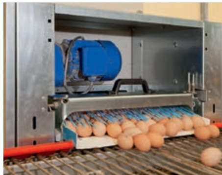
Transfer unit with tension-adjustable wires made from stainless steel (optional)
