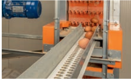
System eggs being transferred to the elevator
