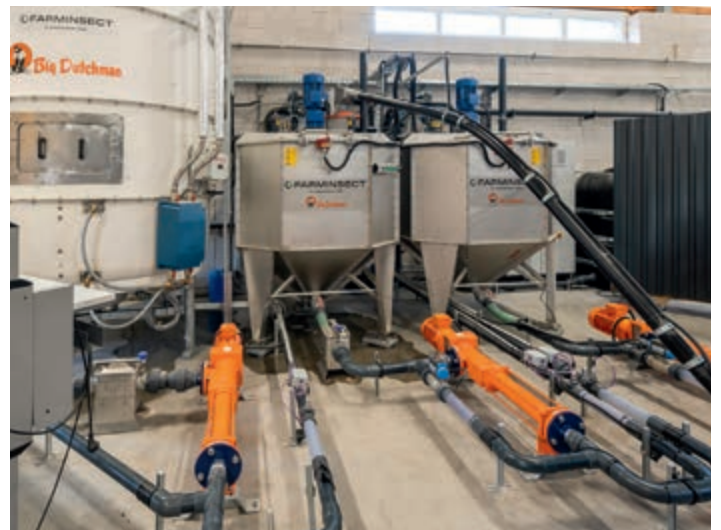
The feed is mixed in two mixing tanks, controlled by a computer. Both tanks are placed on load cells
