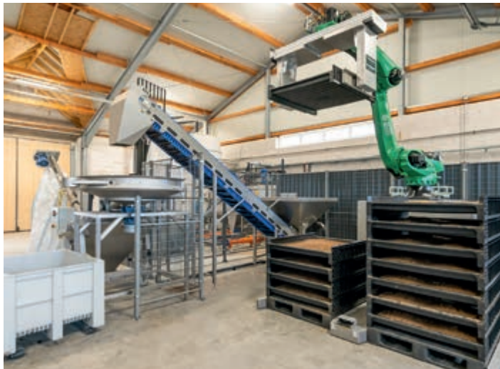
The robot stacks the crates with the feed mix on a pallet, ...
