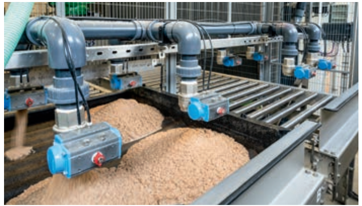
Four feed valves per crate dispense the fresh feed required for one week of larvae growth
