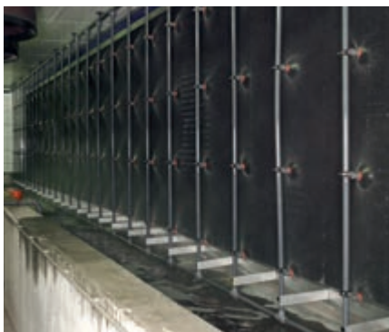
Cleaning stage 1: the filter wall is sprayed with water to prevent dust from adhering
