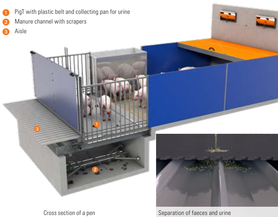
Havito® barn: wean-to-finish system without slurry channels or slatted flooring
