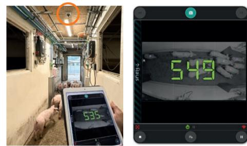
The counted results are displayed in real time on the controller as well as on your smartphone or tablet. For full transparency, you can review a video.
